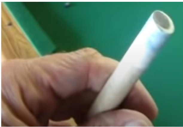
Thoroughly clean the ferrule with rubbing alcohol
