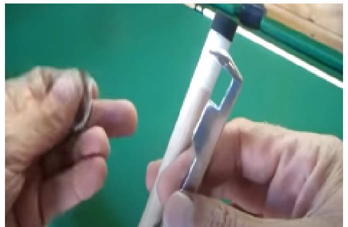
Position the cue clamp in place on the cue shaft (Over the top of the tip)
