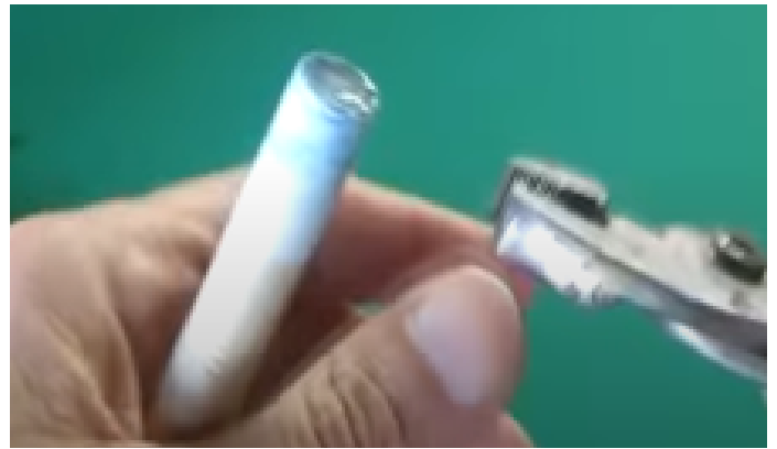
Scuff ferrule top with flat block/180/220 grit sand paper (Keep the ferrule top flat and level)
