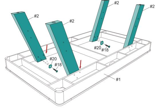
Position the leg on the inside of the support frame and align with pre drilled holes. Insert #18 bolt with #20 washer and loosely tighten in place
