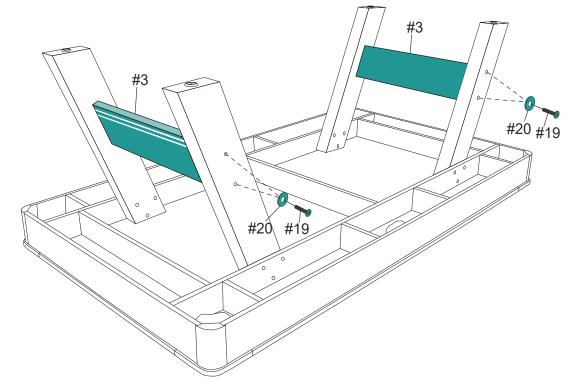
Note: The white design lines on the end leg panels should be facing up when assembling.
