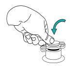
Push cap firmly into the check valve.
